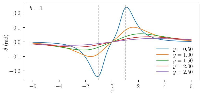
As the slot height, *h*, increases, the peak jet angle increases towards a limiting value. For very large h the jet angle no longer depends on h and so is only a function of the bubble position.
