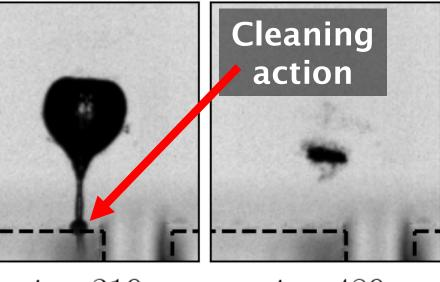
$t = 239 \mu s$  $t = 259 \mu s$  $t = 319\mu s$  $t = 119 \mu s$  $t = 9\mu s$ It is well understood how bubbles collapse near flat boundaries and other simple geometries. However, the understanding of how complex geometries affect bubble collapse is still limited. Here we investigate how a slot geometry affects the collapse of a nearby bubble. The jet can be characterised by a strength and direction. We focus on the jet direction as this can be predicted using very simple models<sup>[2]</sup>.
