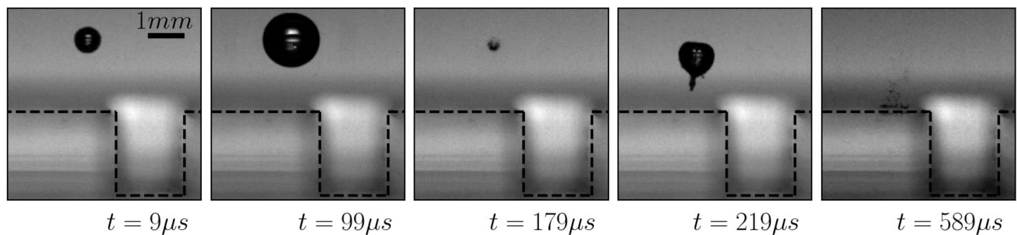
Experiments were recorded at 100,000 frames per second using a high speed camera. This movie shows a negative jet angle, away from the slot, which is also shown by the blue area in the "Numerical Model" plot.
